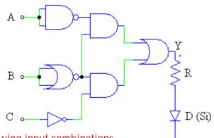
Diode ON in one of three following input combinations such as 000, 001, 100. R = (5 - 0.7) / 2mA = 2,15 K $\Omega$
